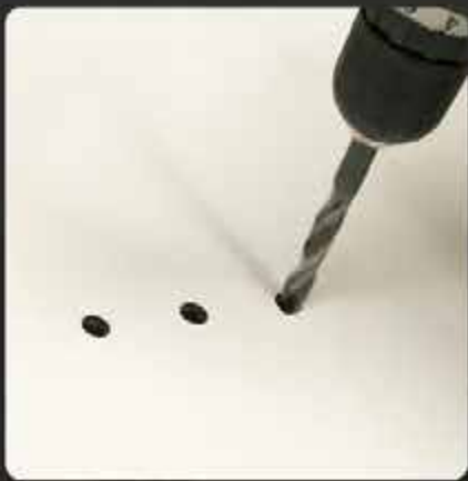
Step 1 Drill mounting holes
